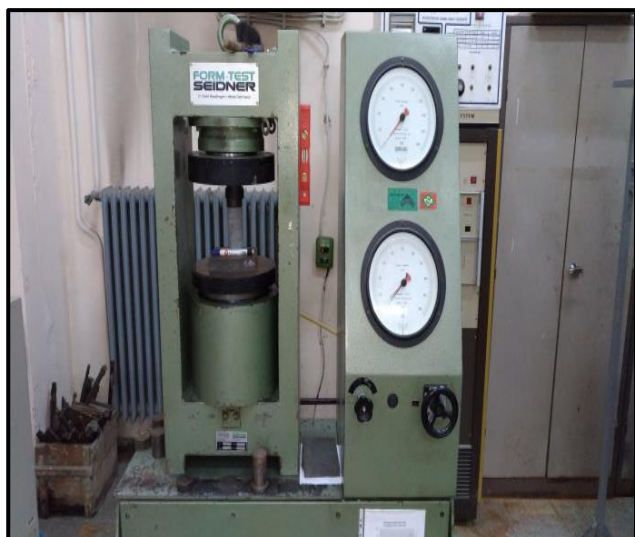
Figure 2. Uniaxial compressive strength testing apparatus.
