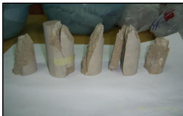
Figure 1. Samples used in uniaxial compressive strength testing.
