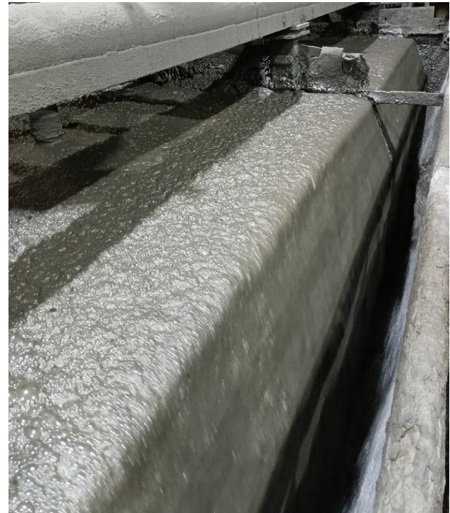
Figure 6. State of the foam when Tomamine and KEX are used
