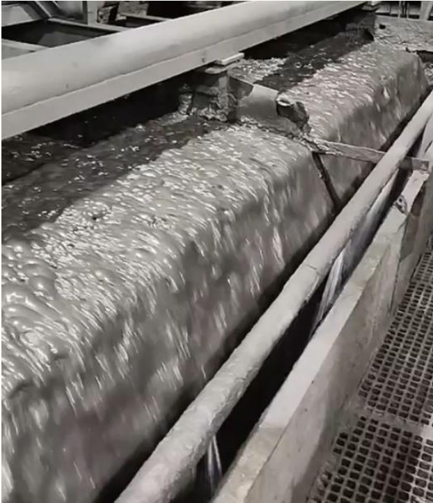
Figure 4. State of the foam when Sodium Butyl Xanthate is used alone
