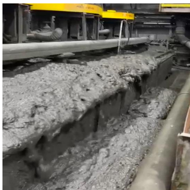
Figure 3. The state of the foam after an overdose of Tomamine M73
