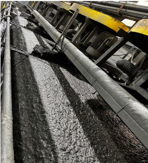
Figure 5. State of the foam when Sodium Butyl Xanthate and Oreprep X133 are used together
