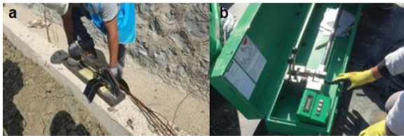
Figure 9. a) Preparation of geomembrane samples before testing, b) Shear test application [20].
