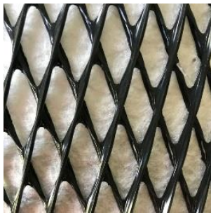
Figure 4. Bottom drainage geocomposite [15].
